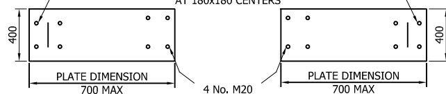
4 No. M20 THREADED HOLES BASEPLATE DRILL & TAPPED FOR LIFTING EYE
