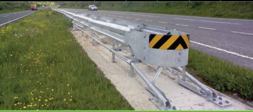
The Quest® CEN system consists of a series of W-beam fender panels supported by diaphragms, and features an integrated front trigger mechanism. The system has been successfully tested using EN 1317-3 criteria for 110 km/h, 100 km/h and 80 km/h levels as a redirective, bi-directional crash cushion.
